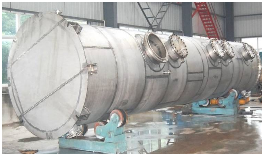
脱氯塔 De-chlorine Tower Material: TA2 (Gr.2) Size: DN2200×10100
