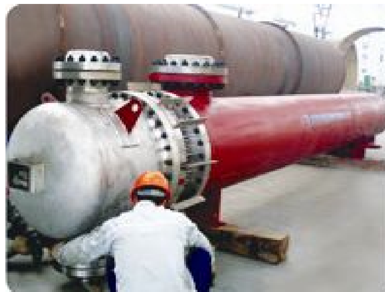
激冷器（双管板）Chiller (Double tube-sheet)
