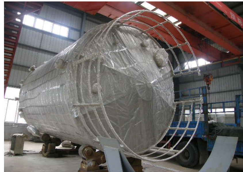
烧碱中间罐 Soda Intermediate Tank
