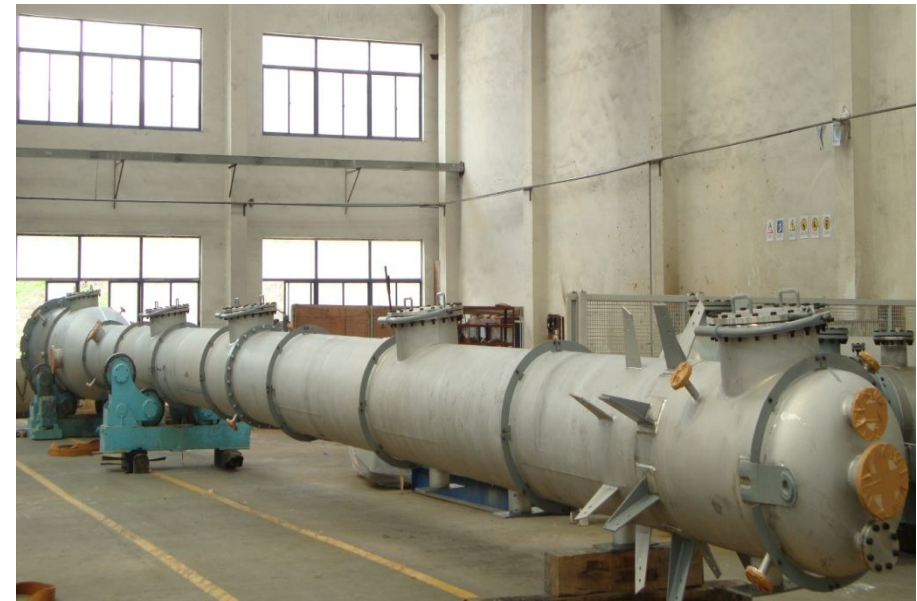
醋酸浓缩塔 Acetic Acid Concentration Tower Material: TA2+Q345R (Gr.2+CS) Size: DN1200×27000
