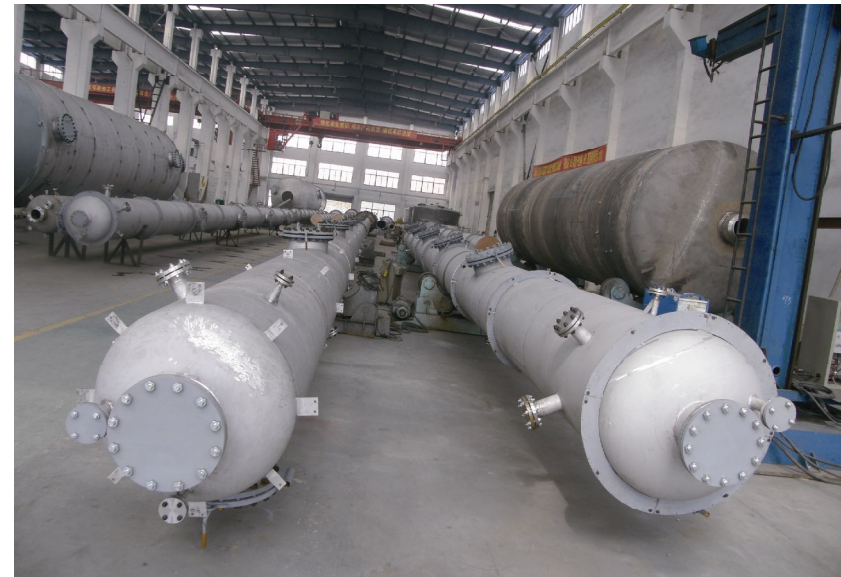
精馏塔 Distillation Tower
