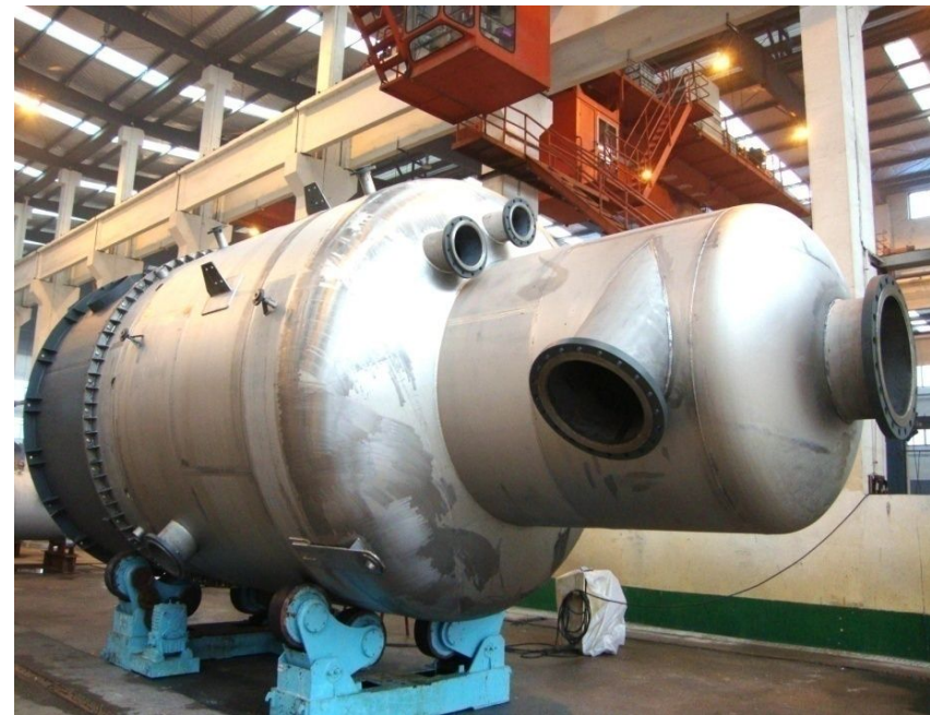
淡盐水储罐 Light Brine Storage Tank
