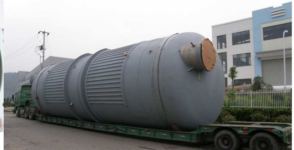
精制塔釜再沸器 Tower Re-boiler Material: 316L+Q345R (316L+CS) Size: DN4600 × 20000
