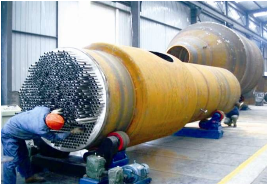
II 效换热器 II-effect Heat Exchanger
