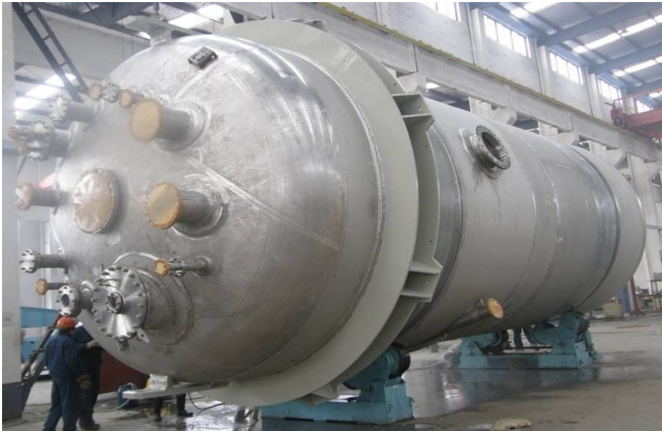
乳胶液泄压罐 Latex Solution Relief Tank
