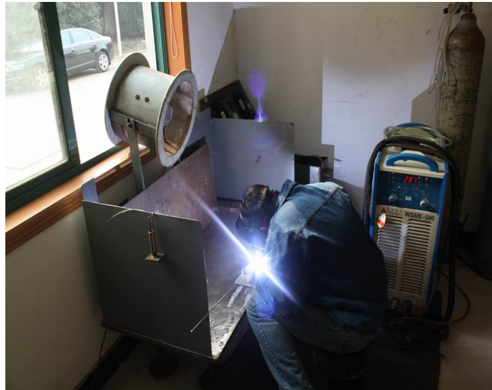
► 焊接试样 Welding Sample
