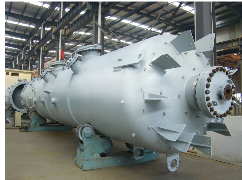
1#丙烯净化槽 1#Propene Refine Tank Material: 09MnNiDR Size: DN2500×15000 NW=70T
