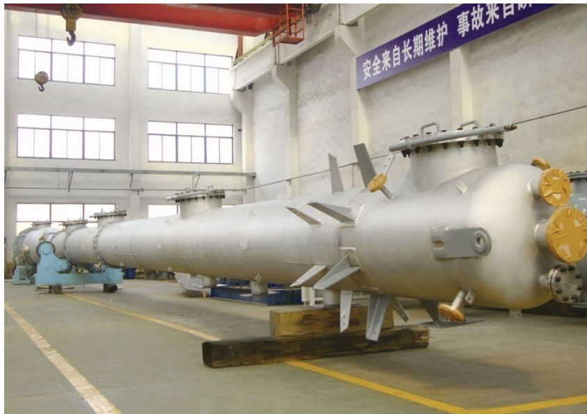
再生塔 Re-generation Tower
