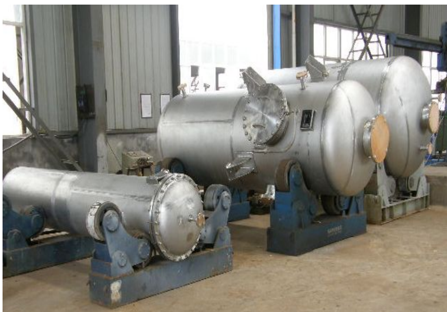
塔回流罐 Tower Re-flux Tank
