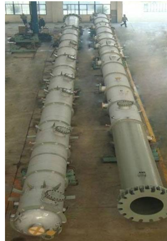
汽提塔 Stripping Tower
