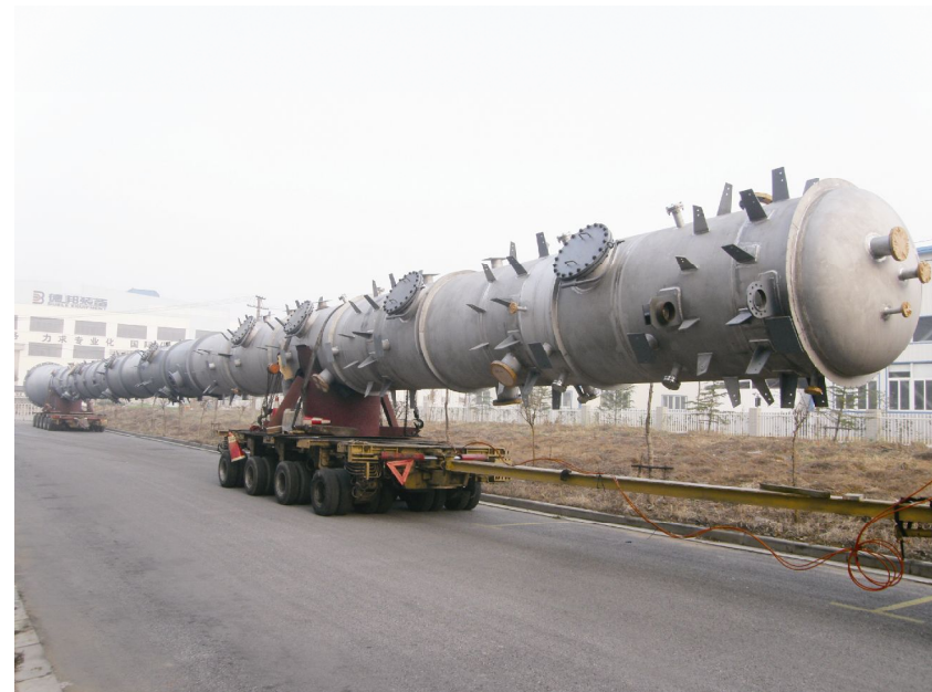
T220再生塔 Regeneration tower
