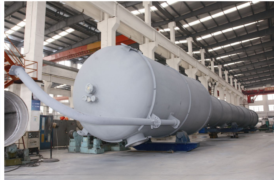
甲醇萃取塔 Extracting Tower Material: 06Cr18Ni11Ti+Q345R(304L+CS) Size: DN2800 × 33000
