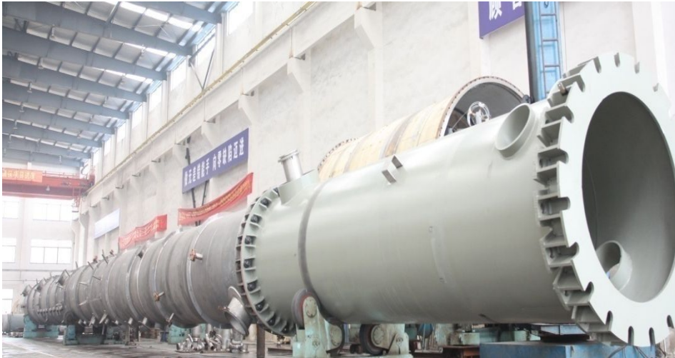
共沸塔: Boiler Tower Material: TA2 (Gr.2) Size: DN2400 × 50000
