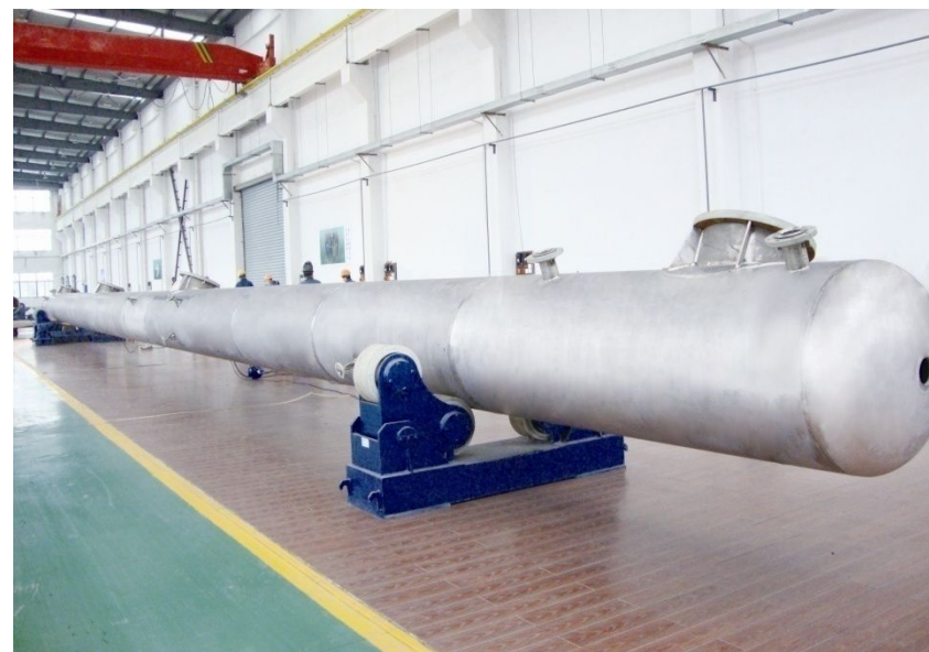
精馏塔 Distillation Tower
