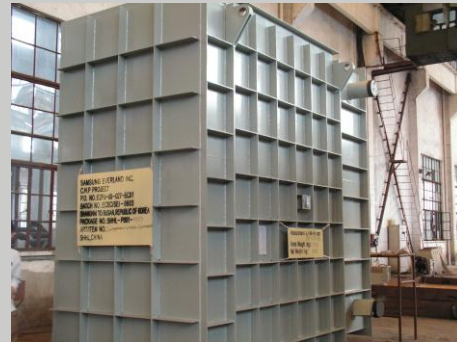
低温过热器 Low temperature superheater
